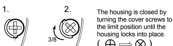
The housing is closed by turning the cover screws to the limit position until the housing locks into place.
